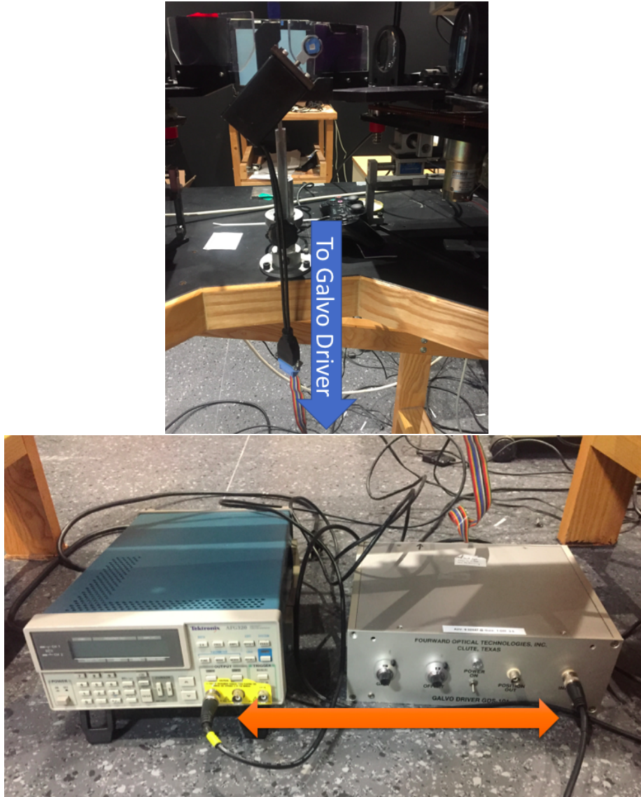
Figure 4: Function generator (left) → galvo driver (right) → galvo with artificial eye (top). The galvo driver should be set with gain 1 and offset 3.5 (written on label). There are two power switches on the galvo driver - one on the front and one on the back to power the galvo. For basic instructions on how to operate the function generator visit the Tektronix manual (page 2-14).
