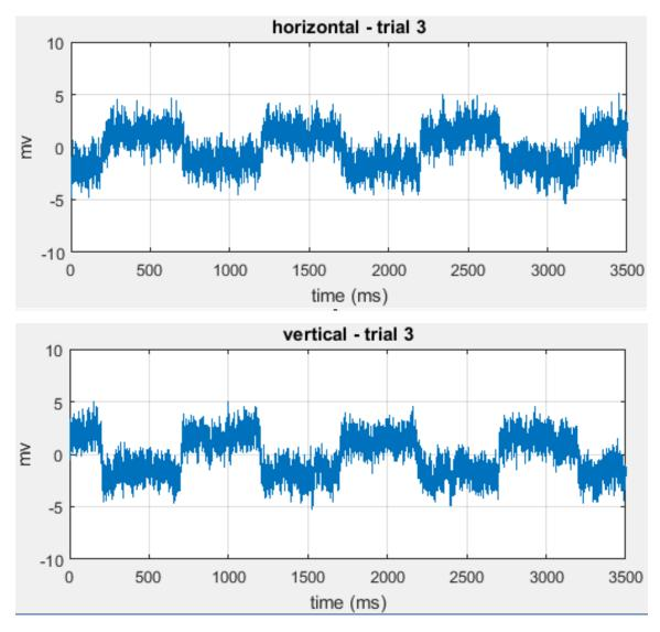
Resolution test at 11:37AM (square 0.1V 1Hz)
