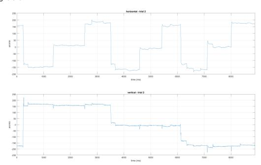
The overshoots don't look right though – sometimes they are missing (example around 2550ms on the left) and they generally decay very slowly (around 2800ms on the right). The oscillations in the vertical trace seem to periodic to us but it could just be the noise level of the vertical system right now.
